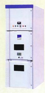
The enclosure of the switchgear is made of high quality—sheet—steel with modular construction. The compartmentalized design of the panel provides isolation between Breaker compartment, busbar compartment, cable compartment and metering compartment. The —compartments are provided with pressure relief passages for safety.
